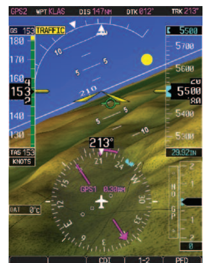
Using familiar TCAS/TAS/TIS symbology in a 3-D format, optional Garmin SVT makes it easier to spot moving traffic. You can see if they're above or below your altitude. And as intruders get closer, the symbols get larger.
