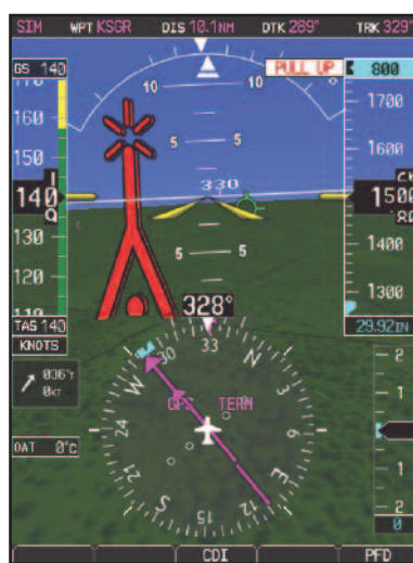
When visibility is low, it's reassuring to have Garmin's Towers and Obstacles database looking out for non-terrain structural hazards. Color-coded 3-D symbols are depicted with SVT to indicate relative proximity of vertical obstruction.
